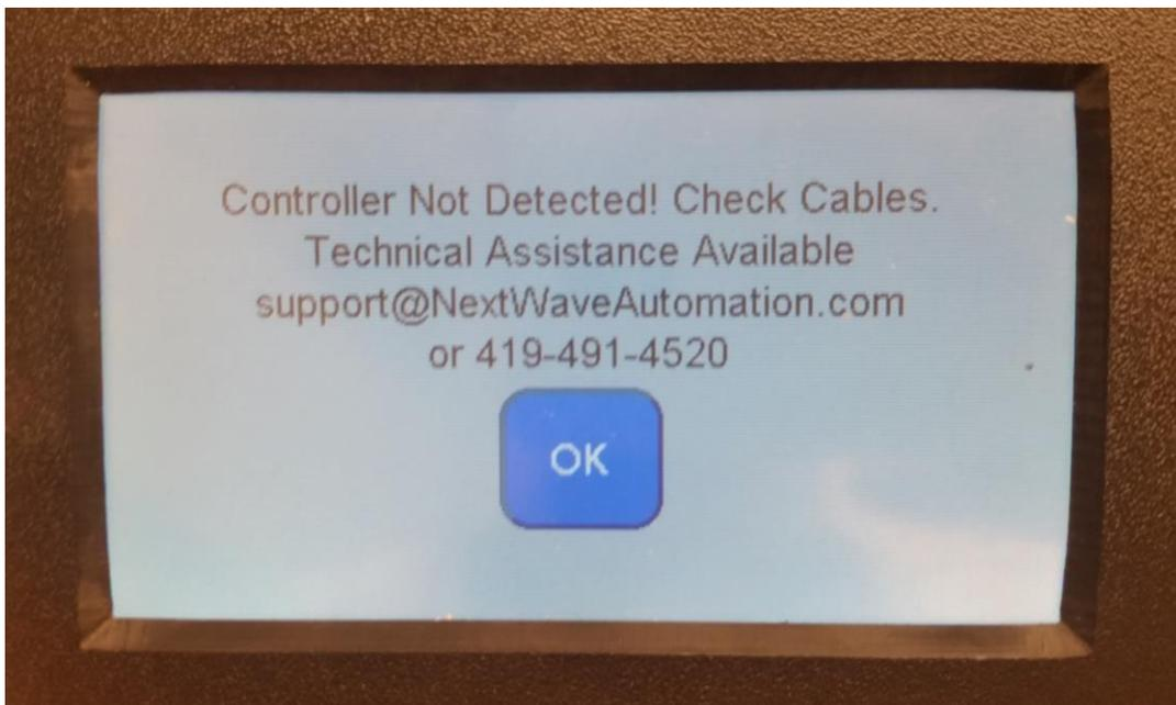
Possible Solution: Turn off your CNC Controller. Ensure that the cable between the LCD Pendant and the CNC Controller is secured on both ends. Ensure that the Touch Probe is not plugged into the CNC Controller. Turn your CNC Controller on. Then plug the probe into the controller, not into the LCD Pendant.
