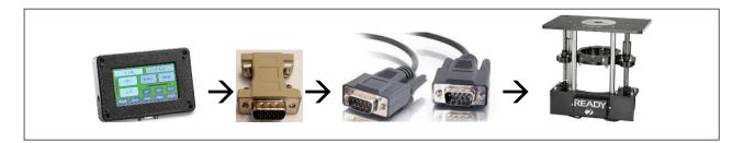
**LIFT Only Configuration: Plug power supply into LIFT** The LCD can be connected directly to the LIFT using a 15:9 pin adapter and DB9M-M Cable
