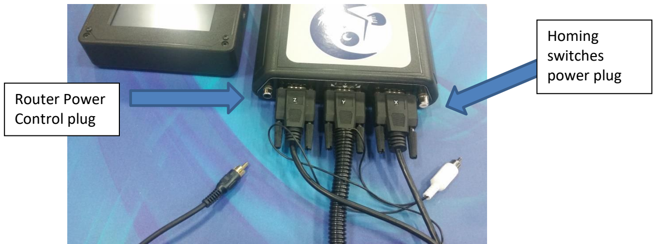
Attaching cables to the back of the Piranha XL controller
