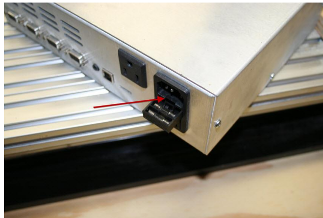
Shark Control Box Power Cord Fuse
