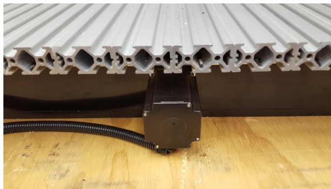
'Front' of Machine - Integrated Base Unit with Y-axis Motor
