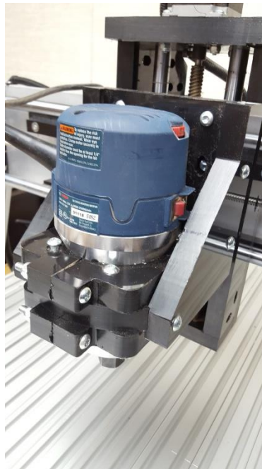
Router Collar and Locking Bolt
