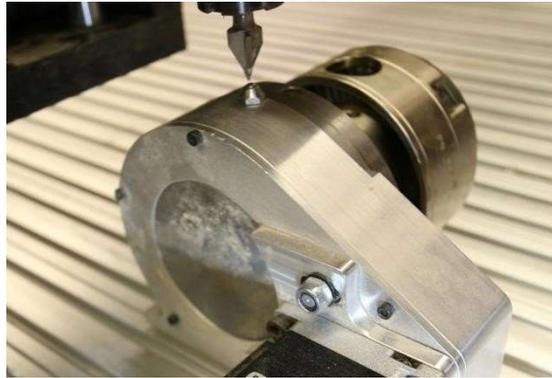
Positioning Along Centerline for X or Y Axis Configuration
