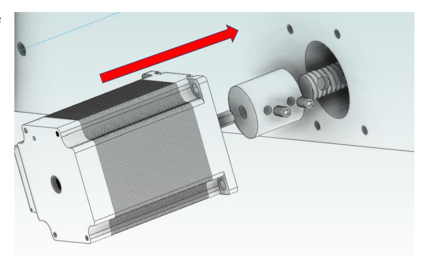
Push the assembled motor, coupler, and threaded rod into the gantry leg.
