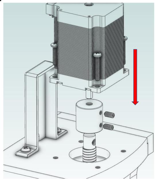
Push the assembled motor, coupler, and threaded rod into the Xbox Assembly.
