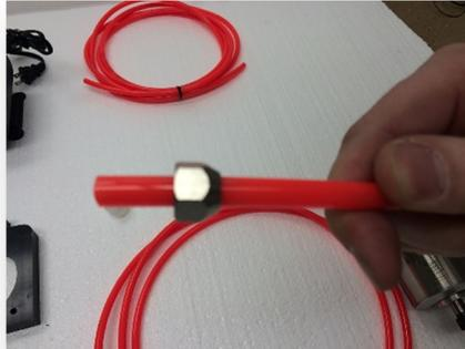
4. Take the orange hose and push it down over the spout that the metal screw head came off of. This should be a very tight fit and to make putting the hose on easier we suggest warming the end of the hose with a heat gun. Be careful not to actually overheat and melt the plastic tube.
