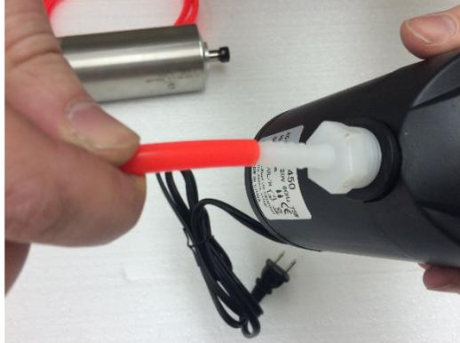
7. Now take the power input cord from the inverter and plug it into the spindle. There will be a groove on the plug that come off the inverter that coordinates with a tongue on the socket of the spindle. Make sure to watch for this to ensure a proper connection. The plug will not fit if these are not matched up.
