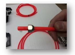
4. Take the orange hose and push it down over the spout that the metal screw head came off of. This should be a very tight fit and to make putting the hose on easier we suggest warming the end of the hose with a heat gun. Be careful not to actually overhear and melt the plastic tube.
