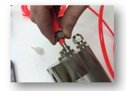
5. Once the end of the hose has been secured onto the spout you can slide the metal screw head down over the hose and spout and tighten it back into place using a wrench.
